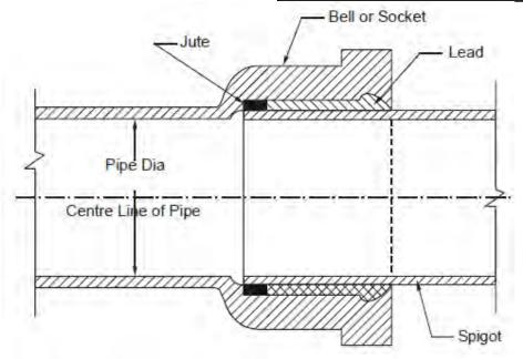
The joint is somewhat flexible and allows the pipe to be laid on flat curves without the use of special mountings. Mostly mains and sub-mains of cast iron, spun iron or steel are joined with this type of joint.
