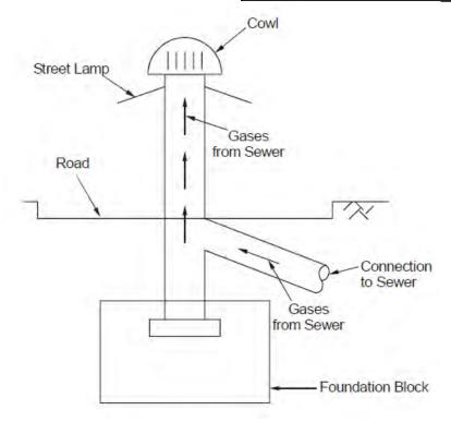
Pressures in the system are developed by the wind blowing up the outlet: and. also by the trapping of air due to surcharge of sewer: and due to other causes as well.
