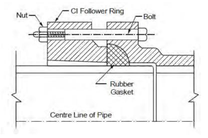
A small gap is kept between the face of the spigot and inner face of the socket. A rubber gasket is provided between the socket and spigot and finally they are tightened with nut and bolt.
